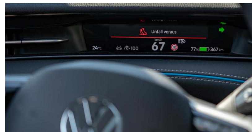
C-ITS Accident Warning in Volkswagen ID.7
